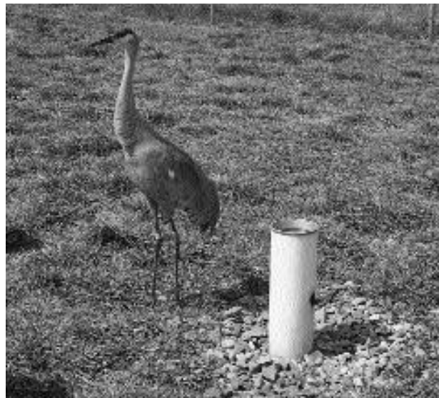
Fig. 12.13. A specially fabricated stainless steel VanEs water cup (15 cm x 15 cm) and Sandhill Crane. Water rises from a supply line at the base of an inverted cone, and drains through holes at water line. Each supply line has a valve accessible through the drain line.
