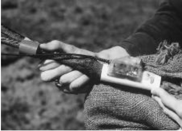
Fig. 11D.6. Radio transmitter on leg band.
